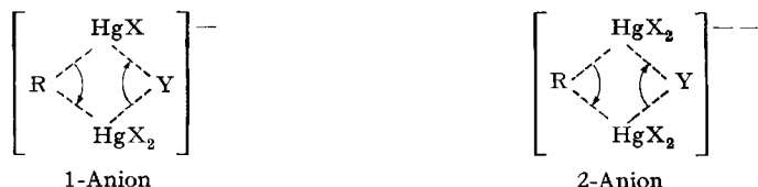
Chart 13. Transition states ( S_{Ei} -type) for 1-anion and 2-anion catalysis of 1-alkyl mercury exchange
